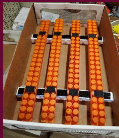
Figure 5. Velcro® strip (10 lb. strength) on the underside of JZs BZs shipping bars to attach to custom shipping bar inserts.
