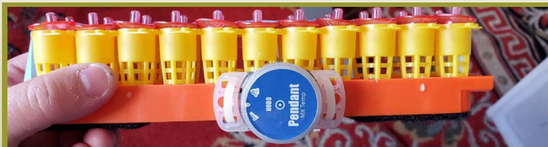
Figure 15. An Onset HOBO Pendant® MX2201 temperature data logger attached to a JZs BZs shipping bar.
