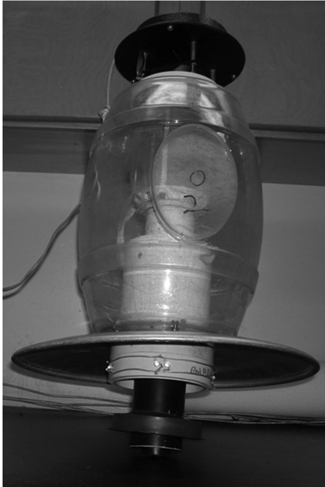
Fig. 2. Mosquito Magnet-X trap modified for reflected light that was used for collection of Lutzomyia spp.
