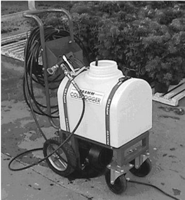
Figure 6. The DRAMM Coldfogger sprayer for greenhouse pest management. The sprayer delivers a fine mist under high pressure.
