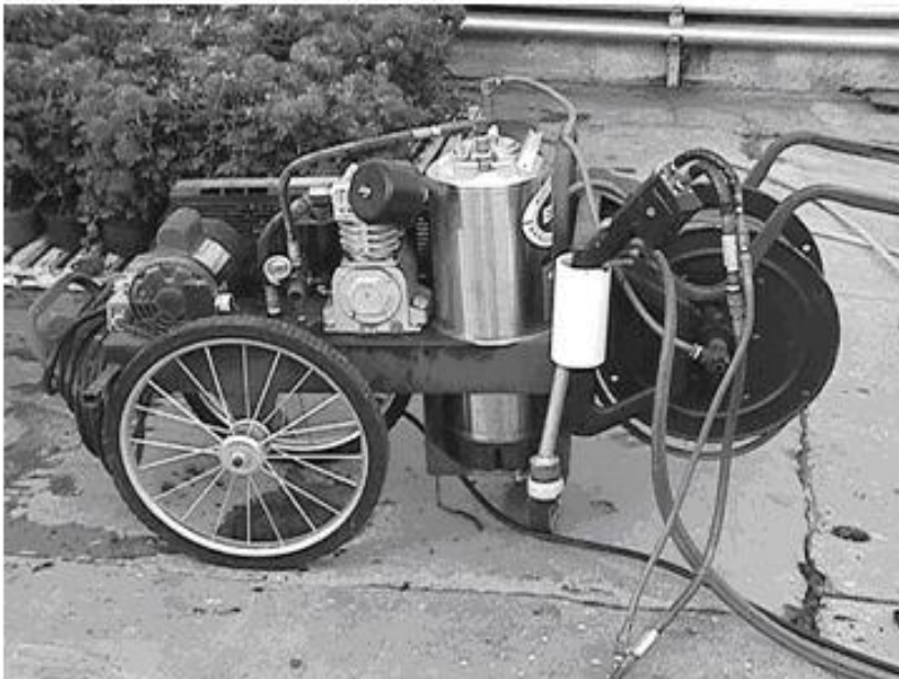
Figure 7. The Electrostatic Spraying Systems Inc. EPS-5 sprayer. The sprayer delivers a fine mist that is electrically charged and forced into the canopy by compressed air.
