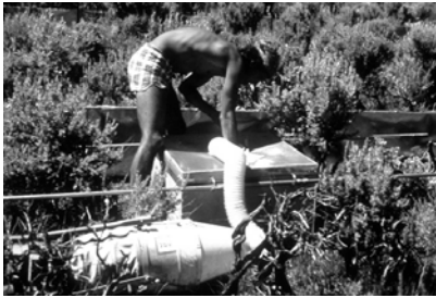
Here a vacuum sampler is used to vacuum the contents of a box placed over shrubs. This effectively converts its operation from a relative to an absolute sampling procedure.
