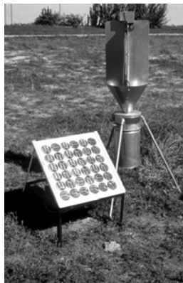
Traps are widely used for insect sampling and monitoring. Light traps (shown here) were more popular before the advent of pheromones. They have the advantage, and disadvantage, of being fairly non-selective. They can be operated off battery or household current. Here the battery is being recharged by a solar panel.
