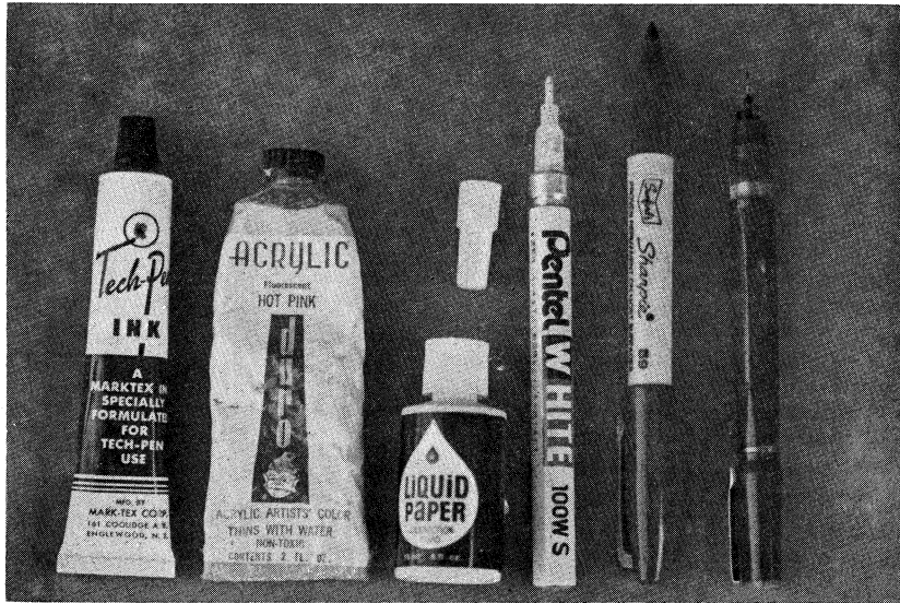
Fig. 2. Some especially useful marking materials (left to right) Tech-Pen “ink,” developed for marking laboratory glassware, is a thick paint that comes in 11 colors 6 ; acrylic paint with day-light fluorescent pigments 7 (acrylics can be thinned with water but are waterproof when dry); Liquid Paper ® correction fluid comes in 9 colors 8 ; Pentel pens deliver a fine line of opaque-white, oil-base ink that dries quickly 9 ; Sharpie ® marking pens have “fine” or “extra fine” points that deliver quick-drying, water-resistant inks (8 colors available) 10 ; technical pens 11 filled with india ink produce uniform lines or dots that can be applied to transparent wings or blots of Liquid Paper (Fig. 3H).
