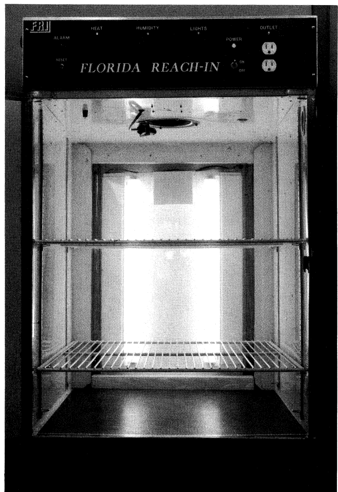
Fig. 2. Open Florida Reach-In, showing control panel with indicator lights and auxiliary outlet, adjustable shelves, lights behind Plexiglas in back, and perforated floor. Sensors for temperature and humidity are in cylinder in air return at center of work space ceiling. Access port, sealed with neoprene stopper, is at upper front of right wall.
