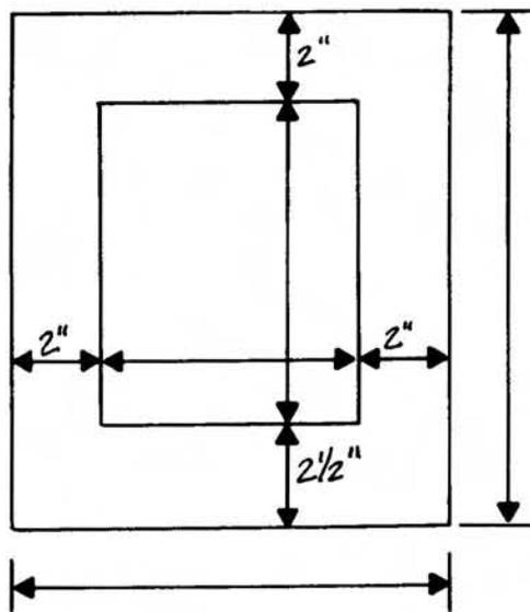
**Figure 11.** Measuring and cutting mats.
